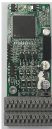
Multi-function incremental PG card EC-PG505-12
