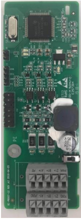
Simplified incremental PG card EC-PG507-12
