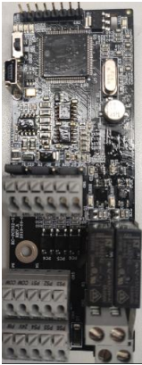
Programmable expansion card EC-PC502-00
