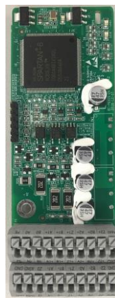
24V incremental PG card EC-PG505-24
