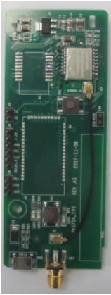
Bluetooth/WIFI communication card EC-TX501/502
