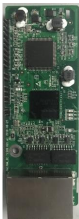
PROFINET communication card EC-TX509
