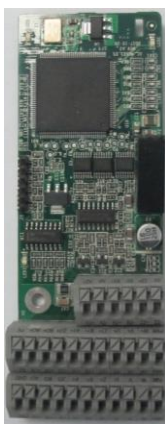
UVW incremental PG card EC-PG503-05
