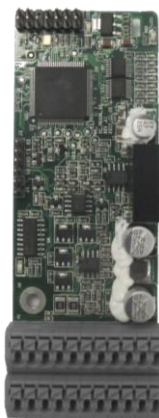
Resolver PG card EC-PG504-00
