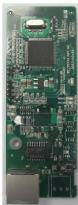
Ethernet communication card EC-TX504
