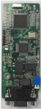
PROFIBUS-DP communication card EC-TX503
