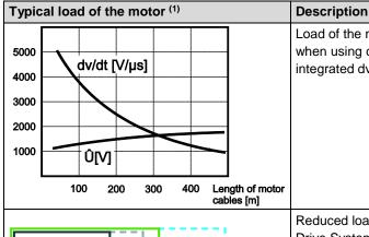
Load of the motor with overvoltage and slew rate when using conventional frequency inverters without integrated dv/dt filter chokes.
