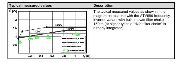
Motors according IEC 60034-25 as well as motors according NEMA MG1 are dimensioned for operation with frequency inverters and thus they are well qualified for drives with ATV680 frequency inverters.
