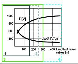
Reduced load of the motor by using Altivar Process Drive Systems with integrated dv/dt filter chokes 150 m (at higher types a "dv/dt filter choke" is already integrated).
