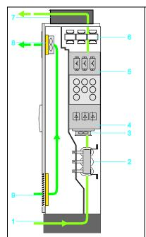
In case of increased protection degree IP54 with separate air channel the cooling air inflow for the power part takes place through the floor and the air outlet through the enclosure roof. The control part is cooled by filter fans in the enclosure door.
