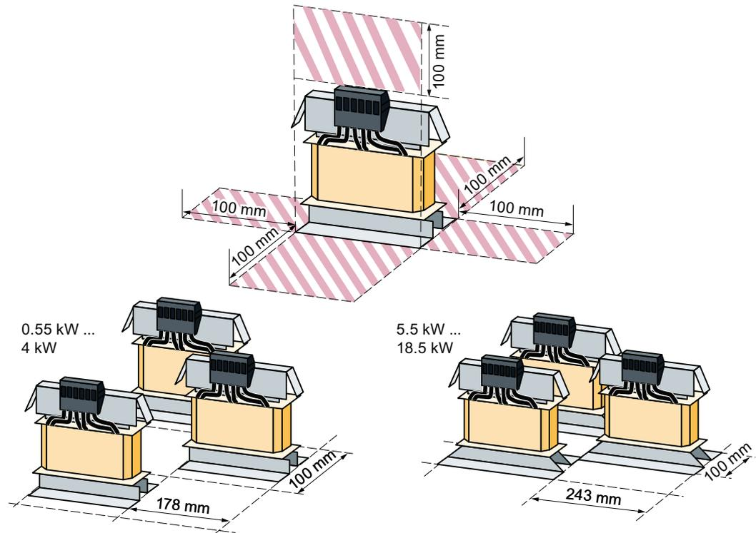
Figure 8-5 Minimum clearances of the output reactor to other devices, space-saving mounting examples
