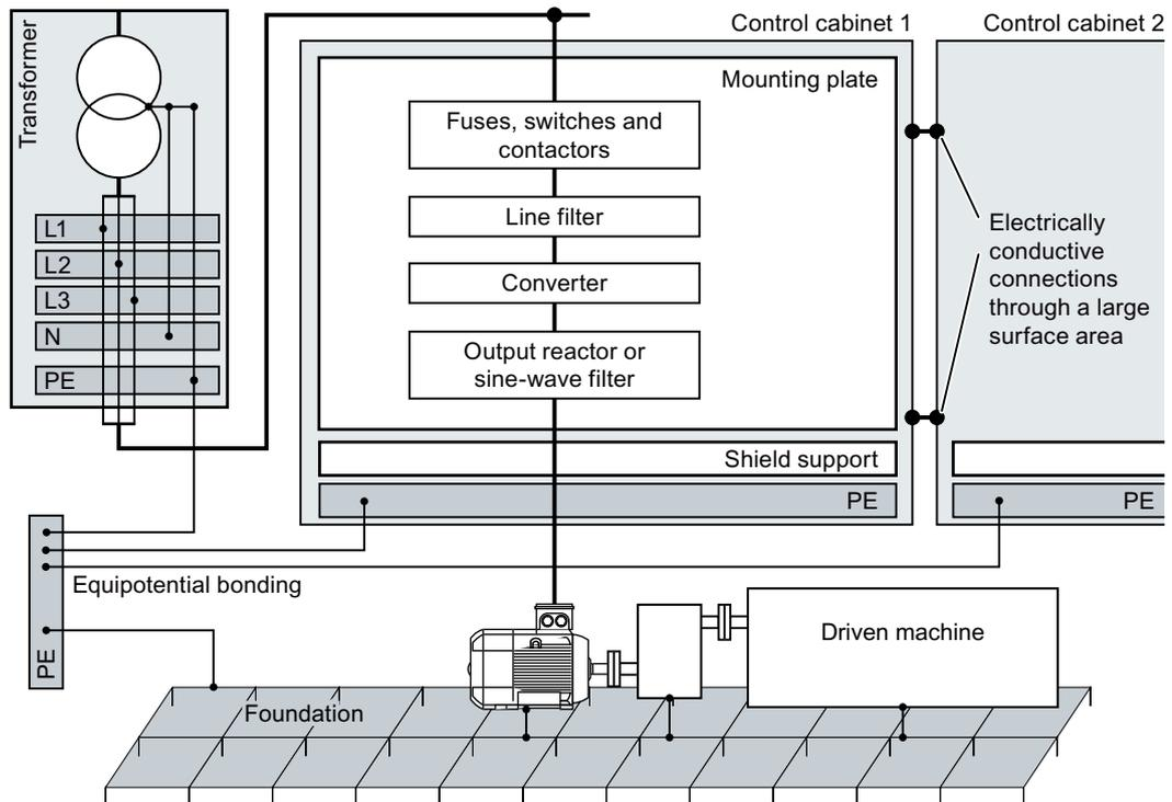
Figure 4-4 Grounding and high-frequency equipotential bonding measures in the control cabinet and in the plant/system
