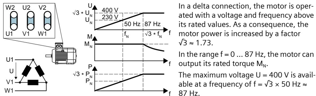
The motor only goes into field weakening above 87 Hz.
