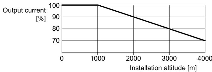
Figure 7-2 Current derating as a function of the installation altitude
