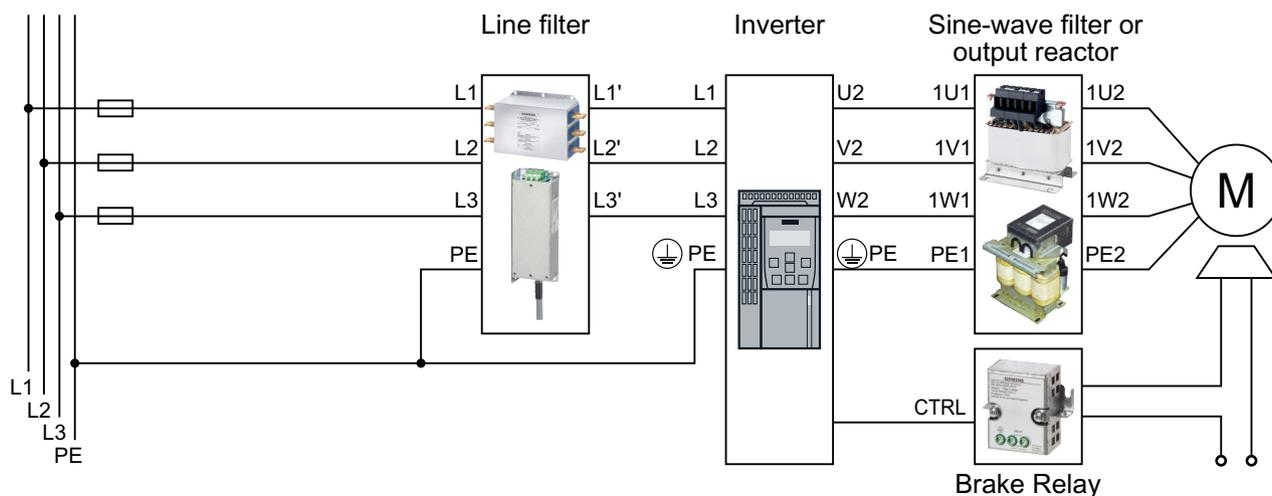
The converters are available with or without integrated line filter (category C2). There are external filters (category C1) for increased EMC requirements for frame size FSC.
