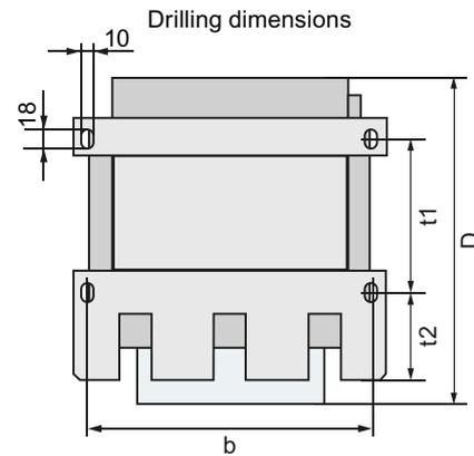
Figure 8-10 Dimensions - standalone filter
