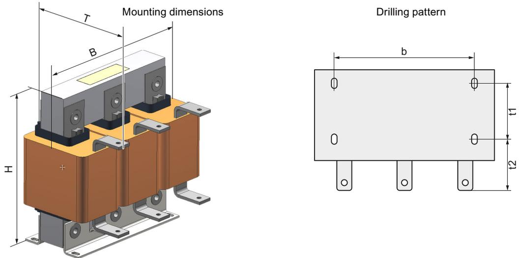
Figure 8-7 Standalone output reactor for frame sizes FSD ... FSF
