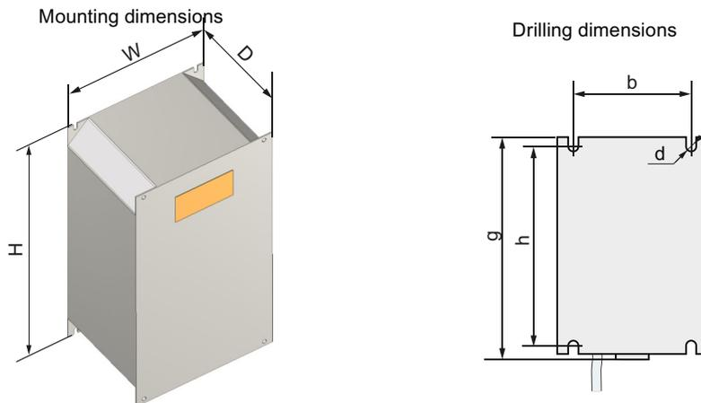
Figure 8-8 Dimensions - footprint filter
