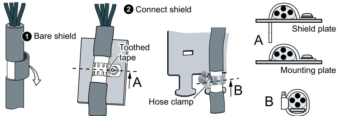
Figure 4-3 Examples for EMC-compliant shield support
