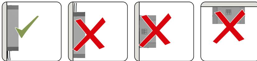
Figure 8-9 Mounting position - footprint filter
