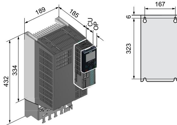
Table 4-1 Dimensions depend on the Control Unit (CU) and Operator Panel (OP)
