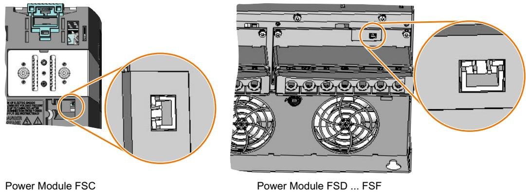
Figure 8-12 Connector position for the Brake Relay
