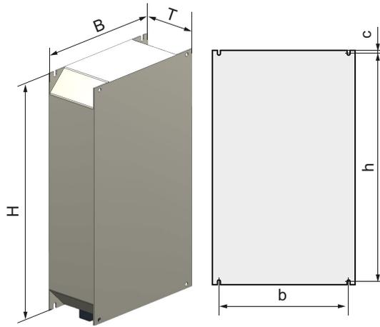
Figure 8-6 Output reactor as base component for frame size FSC
