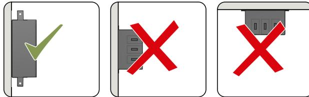
Figure 8-4 Mounting position FSF
