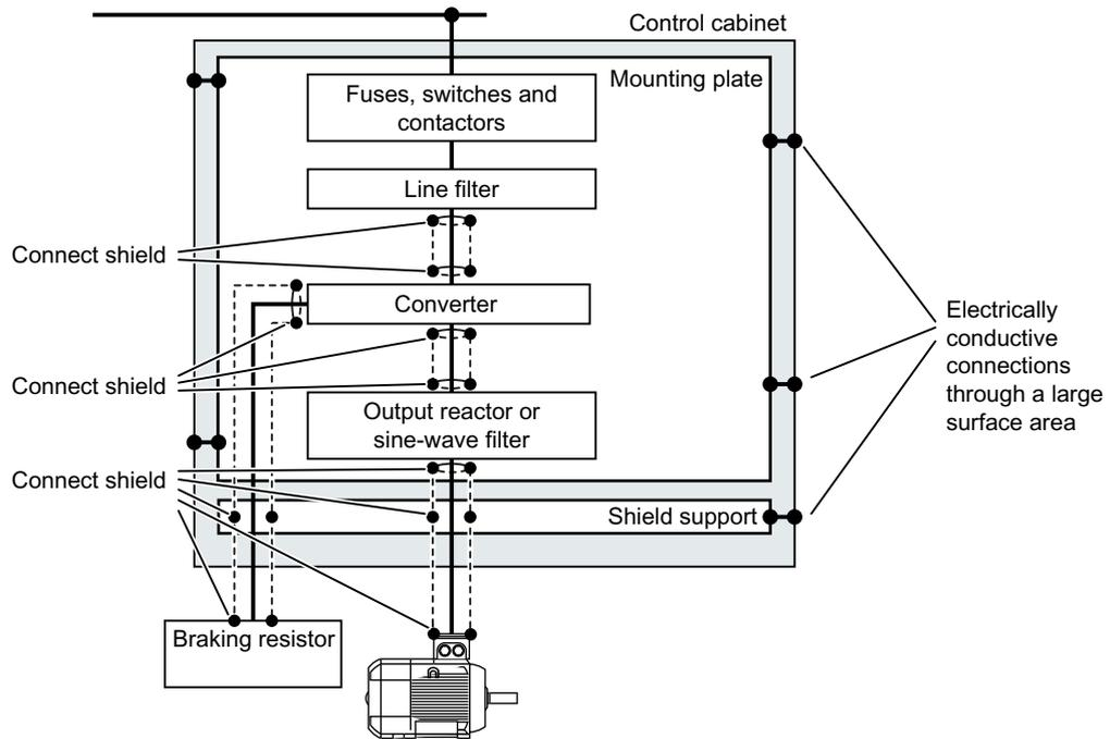
Figure 4-2 Routing converter cables inside and outside a control cabinet
