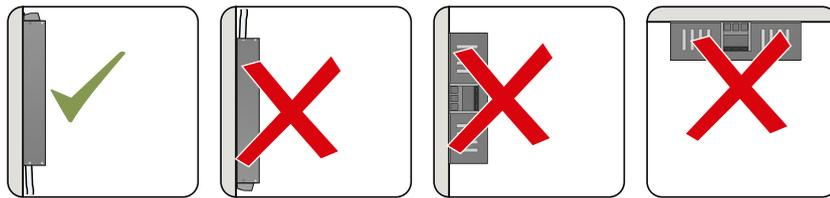
Figure 8-2 Mounting position FSC
