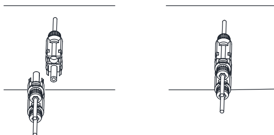
Pic 5.6 DC input connection
