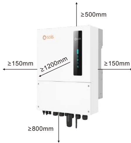
Figure 3.5 Inverter Mounting Clearances
