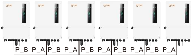
Figure 3.24 Parallel Terminal Connection
