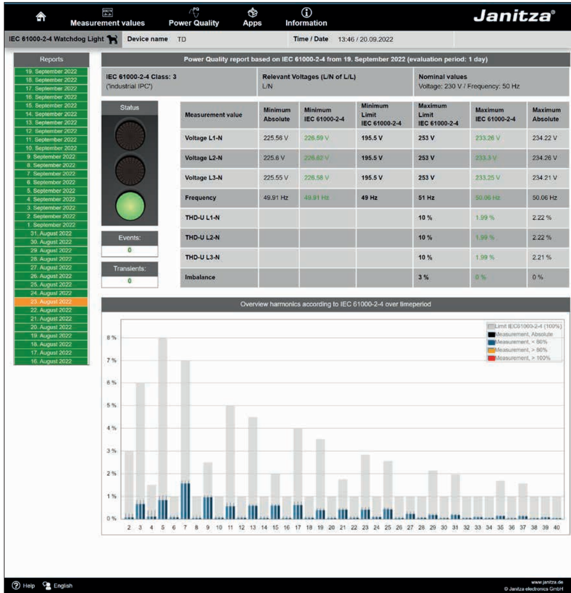
Fig. IEC 61000-2-4 Watchdog parameters with traffic light principle - report
