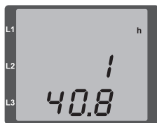
Fig. Operating hours meter of the measured value display
