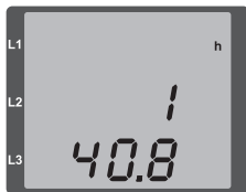
Fig. Measured value indications Operating hours meter The UMG 96RM-E operating hours meter reading is 140.8h. This corresponds to 140 hours and 80 industrial minutes. 100 industrial minutes = 60 minutes. In this example, 80 industrial minutes = 48 minutes.
