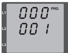
Fig. Programming mode Parameter indication Use button 1 and 2 to change individual parameters (see page 46).
