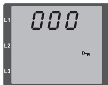
Fig. Password query Use button 1 and 2 to enter a password (if any).
