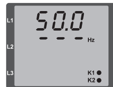
Fig. No rotation field direction detectable.
