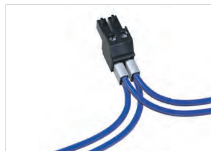
Fig.: 2-pole plug contact with cable connection (cable type: 2 x 0.75 mm 2 ) via twin core end sheathes
