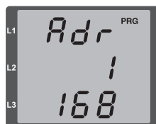
Fig. TCP/IP address, Byte 1 A TCP/IP address consists of 4 bytes with the following structure:
