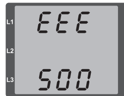
Fig. Warning message with number 500 (mains frequency)
