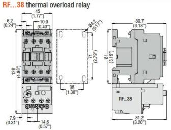
BF26 00A... - BF32 00A... - BF38 00A... three poles with RF...38 thermal overload relay
