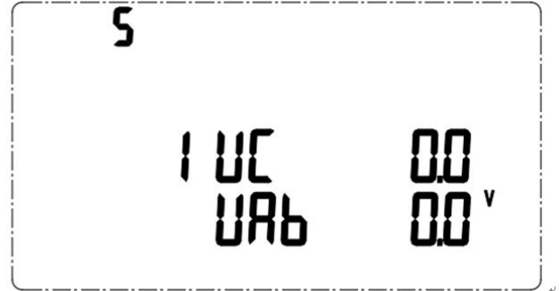
Phase voltage U_c and line voltage U_{ab}
