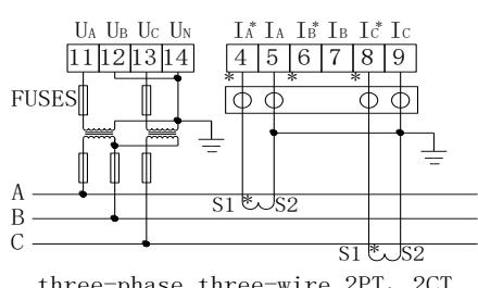
Note: For Three-phase-three-wire, No. 12 terminal must be connected with No.14 terminal
