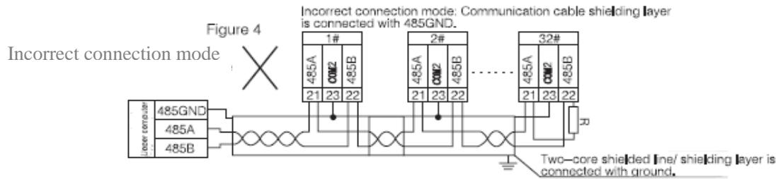
Recommendation of adding matched resistance between A<sub>1</sub> B of the last meter, the rated resistance range is 120Ω~10kΩ.
