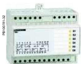
M6C programmable contacts: circuit-breaker external relay with six independent changeover contacts controlled from the circuit breaker via a three-wire connection.
