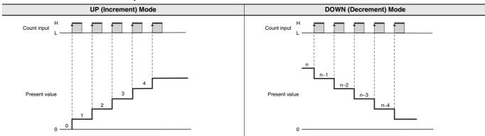
$\boldsymbol{*}$  Counting starts when the count input is turned ON after turning ON the power.
