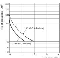
A current of 0.15 A max. can be switched at 125 VDC ( $cos\phi=1$ ) and current of 0.1 A max. can be switched if L/R=7 ms. In both cases, a life of 100,000 operations can be expected.
