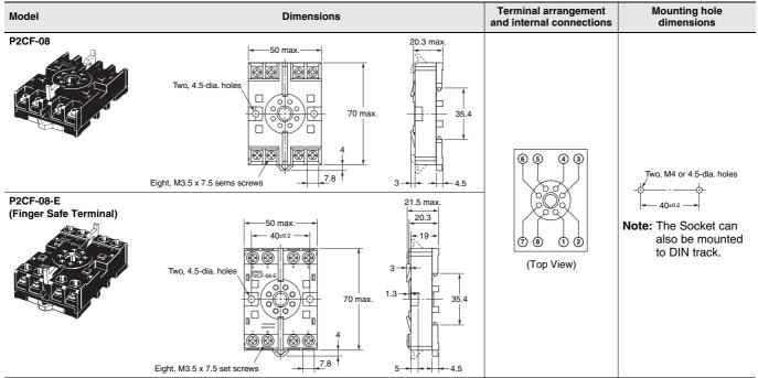
Note: Round crimp terminals cannot be used on Finger-safe Sockets. Use forked crimp terminals.
