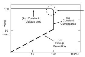
Typical LED power supply I-V curve
