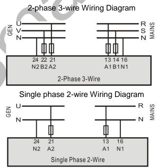
**ANOTE:** Above pictures take the AC 220V voltage as example. If AC 110V voltage is applied in actual use, please contact with Smartgen technical staff to get the specific wiring methods.
