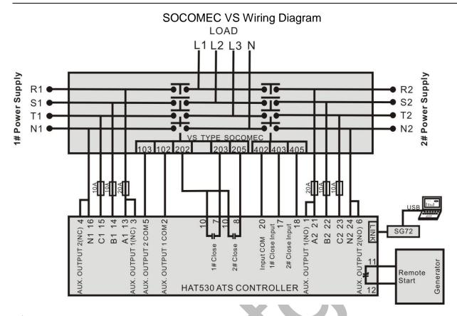
Note: The diagram is for reference only. The actual wiring shall follow the ATS instruction. Users should choose proper fuse capacity according to the actual power consumption. If SOCOMEC VS is applied, the Close delay and Open delay must be no less than 5s (Default: 5s).
