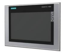
SIMATIC HMI TP900 Comfort INOX Stainless steel front, Continuous decorative film, Degree of protection front IP66K, 9" widescreen TFT display, PROFINET interface, MPI/PROFIBUS DP interface, 12 MB configuration memory, Windows CE 6.0, (Microsoft Support included Security updates discontinued) configurable from WinCC Comfort V11
