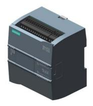
SIMATIC S7-1200, CPU 1211C, compact CPU, DC/DC/DC, onboard I/O: 6 DI 24 V DC; 4 DO 24 V DC; 2 AI 0-10 V DC, Power supply: DC 20.4-28.8V DC, Program/data memory 50 KB
