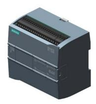
SIMATIC S7-1200, CPU 1214C, compact CPU, DC/DC/relay, onboard I/O: 14 DI 24 V DC; 10 DO relay 2 A; 2 AI 0-10 V DC, Power supply: AC 20.4-28.8V DC, Program/data memory 75 KB
