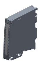
SIMATIC S7-1500, analog output module AQ 2x U/I ST, 16-bit resolution accuracy 0.3%. 2 channels in groups of 2, diagnostics; substitute value; the module supports the safety-oriented shutdown of load groups up to SILCL1 according to EN 62061:2005 + A2:2015, and Category 2 / PL c according to EN ISO 13849-1:2015. delivery including front connector push-in, infeed element, shield bracket and shield terminal
