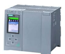
SIMATIC S7-1500, CPU 1517-3 PN/DP, Central processing unit with work memory 2 MB for Program and 8 MB for data, 1st interface: PROFINET IRT with 2-port switch, 2nd interface: PROFINET RT, 3rd interface: PROFIBUS, 2 ns bit performance, SIMATIC Memory Card required
