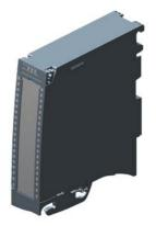
SIMATIC S7-1500, digital output module DQ16x24 V DC/0.5A HF; 16 channels in groups of 8; 4 A per group; single-channel diagnostics; substitute value: switching cycle counter for connected actuators. the module supports the safety-oriented shutdown of load groups up to SILCL2 acc. to EN 62061:2005 + A2:2015, and Category 3 / PL d according to EN ISO 13849-1:2015. front connector (screw terminals or push-in) to be ordered separately
