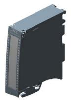
SIMATIC S7-1500, digital output module DQ 32x24V DC/0.5A HF; 32 channels in groups of 8; 4 A per group; single-channel diagnostics; substitute value, switching cycle counter for connected actuators. the module supports the safety-oriented shutdown of load groups up to SILCL2 acc. to EN 62061:2005 + A2:2015, and Category 3 / PL d according to EN ISO 13849-1:2015. front connector (screw terminals or push-in) to be ordered separately
