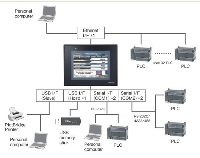
\*1. The Ethernet communication and USB Host are supported only by NBD-TW01.
