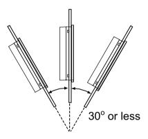
When installing the GP unit in a slanted position with an incline more than 30°, the ambient temperature must not exceed 40 °C (104 °F). You may need to use forced air cooling (fan, A/C) to ensure the ambient operating temperature is 40°C or less (104 °F or less).
