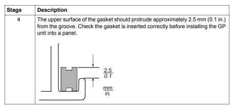
The gasket must be inserted correctly into the groove for IP65F moisture resistance for the GP unit.
